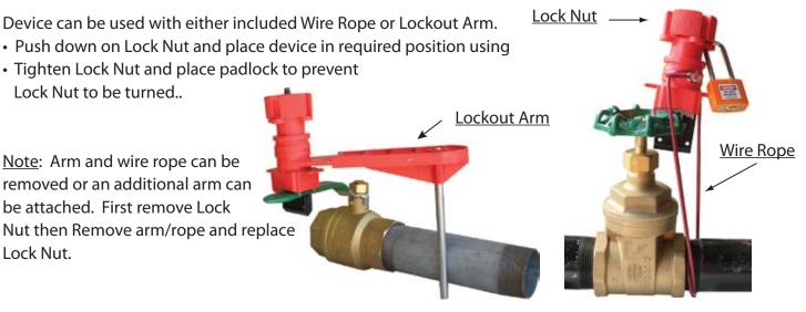
Ensure that device cannot be removed and that access to the valve handle is blocked efficiently so handle cannot be turned. If the device cannot securely hold valve handle in a safe postion - IT MUST NOT BE USED.
